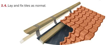
**NOTE:** If at this stage it is acknowledged that the brackets were not set high enough at stage 1, then another batten can be screw fixed on top of the original to achieve correct engagement.
