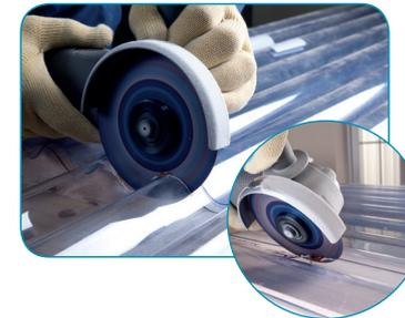
A good tip when cutting, is to sandwich the sheet between other sheets with the part to be removed protruding.
