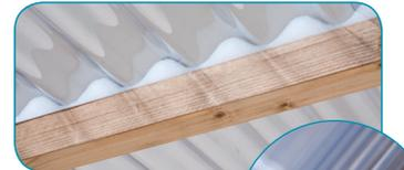
Use Ariel screws, caps and washers to secure the sheet: the screw is sufficiently tight when the washer under its head can just be rotated with finger and thumb.
