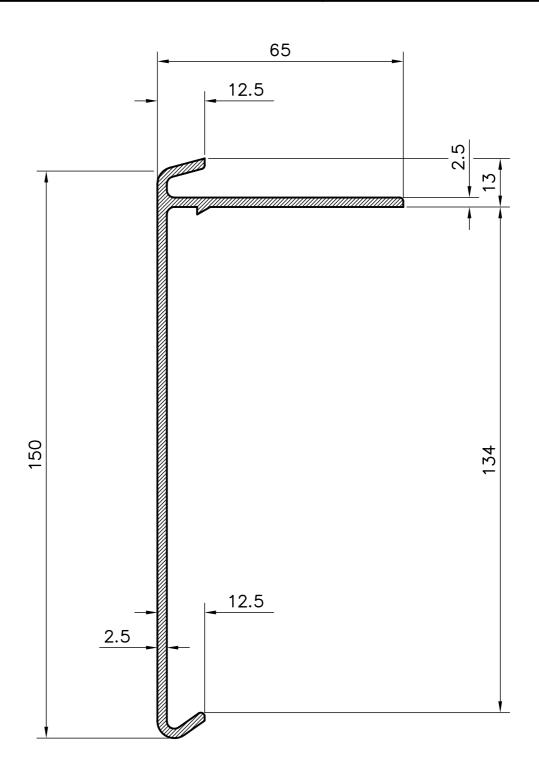
SUPPLIED IN 2.5 METRE LENGTHS WITH LOOSE JOINTING SLEEVE 90° INTERNAL AND EXTERNAL CORNER PIECES AVAILABLE STANDARD COLOURS BLACK, WHITE AND GREY OTHER COLOURS CAN BE SUPPLIED, PRICES & LEAD TIMES ON APPLICATION
