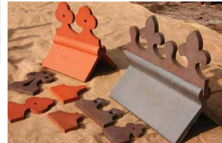
**Right:** These slotted roll top ornamental ridges pictured have a groove in their length to take specially made inserts. These inserts are bedded into the roll using mortar. Any shape of insert can be manufactured and here you can see some examples of various shapes we have made.
