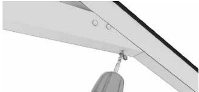
**2** Fix tie bar to rafter by screwing through pre drilled hole in the bottom of the tie bar.
