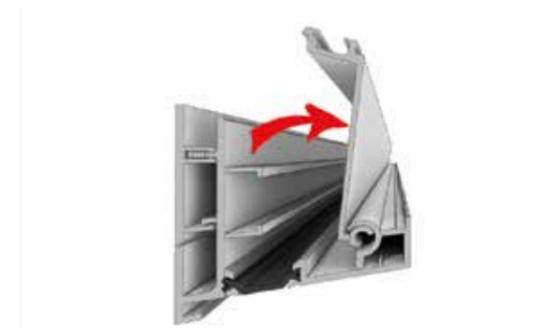
**7** Insert ringbeam flaps by locating hinge part of the flap into the main ringbeam at approx 80 degrees as shown, then rotate forward to lock in.
