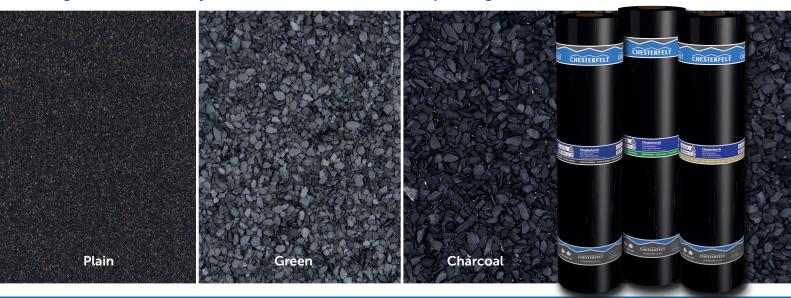
Chestertorch is a multi-layered bituminised waterproof system designed for use on various types of flat roofing projects including new build and refurbishments, cold roofs and warm roofs using vapour control layers with insulation. This range of membranes feature a polyester core which is saturated and coated in modified bitumen and the upper surface is finished with a choice of either light sand or slate mineral.
